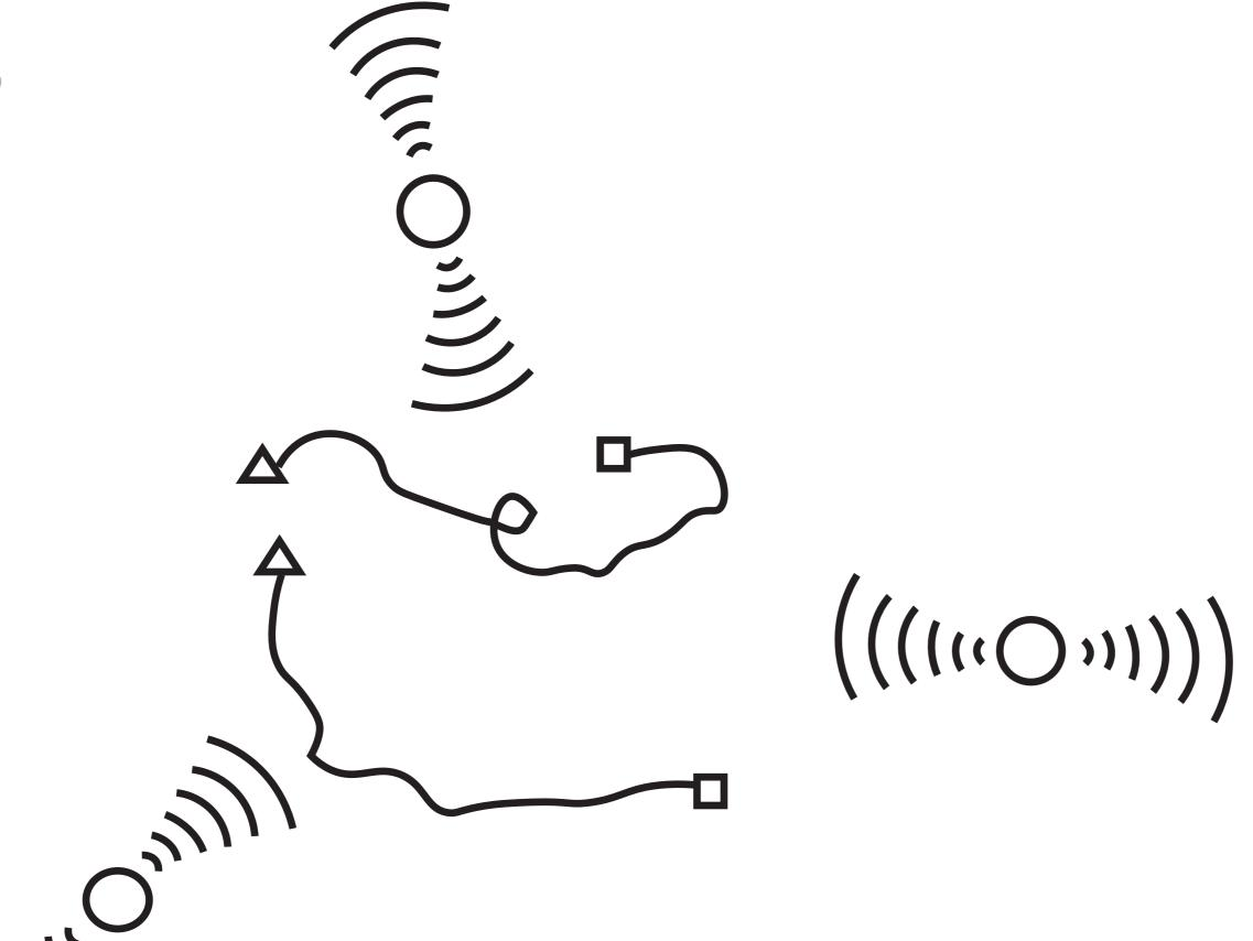
Fig 6. Bird's-eye view of three sound-source moorings (Open Circles) and two float trajectories (squiggly lines). The triangle is where the float was launched, and the square is where the float surfaced.
